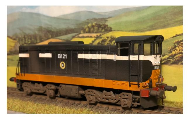
Check clearances by test running through points and curves. Its easier to make corrections now changes now before detailing has been added that would be vulnerable to accidental hand pressure
