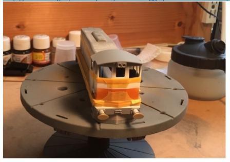
17. Form and Add grab and hail rails around cab doord, cab windws, end of bonnet walkway, face of cab. These can be later hand painted. I used a simple needle nose pliers and a tweezers to for the various metal grab rail components for strips supplied by eileens emphorium.
