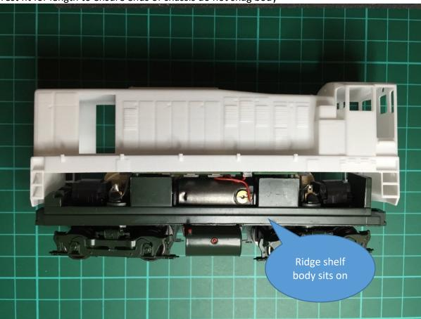
Test fit for length to ensure ends of chassis do not snag body
