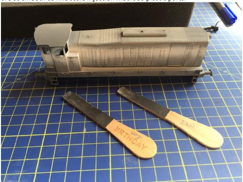
9a. hand drill any holes that will later be need to fit any of the metal grap rails (ie to avoid drill damge after painting.
