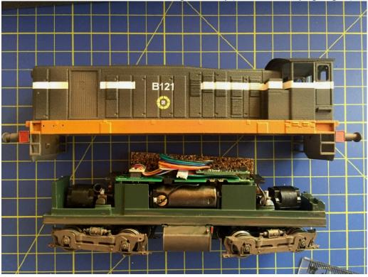
13. Remove Athearn SW1500 fuel tank and replace with plasticard one or modified salvage. Carefully ensure bogie clearance after the GM bogie sides have been added (especially checking the singe brake cylinders clear the fuel tank and the front of the bogies clear the ladder and valance.
