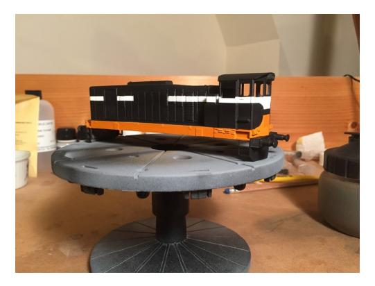
11. Test fit body to chassis. If internal plastic body mounting spacers were neatly cut the body should friction fit nicely (later you can add internal plastic body mounts and screws). I used the Kadee coupling tongs or Tension lock coupling tongs as a means of stopping one end of the body slipping off.
