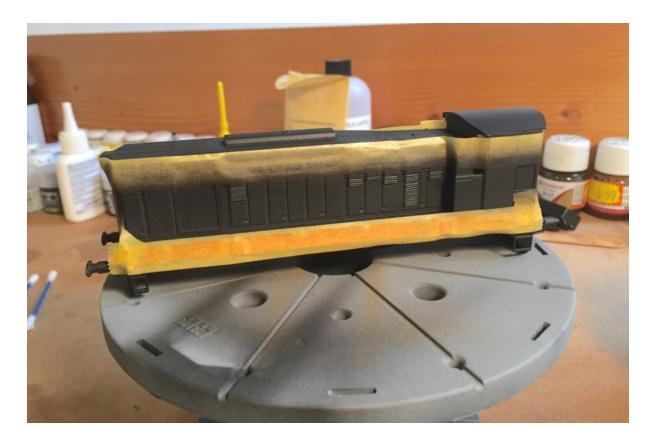
Reverse masking helps get the white bands level with well defined edges. http://www.derg.ie/albums/l278/OceanFroggie/model%20rail%20painting/IMG 1725.jpg
