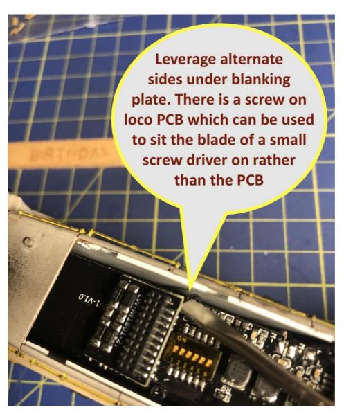
3. The decoder should not cover the dip switches, see photo below, it goes towards the cab end fitting under the panel in front of the cab windows. There are wires in there so it won't fit initially until you nurse it into place easing it gently past the wires
