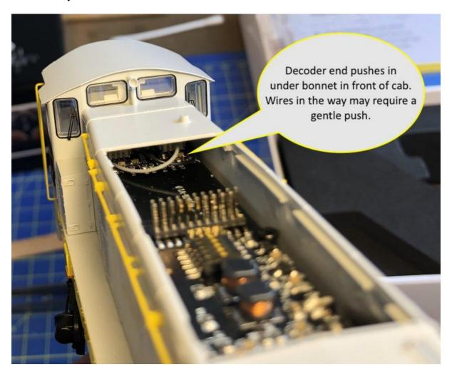
Note the 21pin strip of pins has one missing on the loco PCB and the decoder is missing one hole, this is so that you align the decoder correctly. Be very careful to get this blank hole and missing pin aligned ok, it is very easy to bend pins if one hasn't go this right and force the decoder down. I find the locos pins will fit the decoder loosely giving you a clue its lined up ok before gentle finger pressure to push the decoder down allowing the pins up into the decoder holes.
